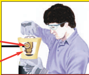
Operator wearing PPE in safe position
