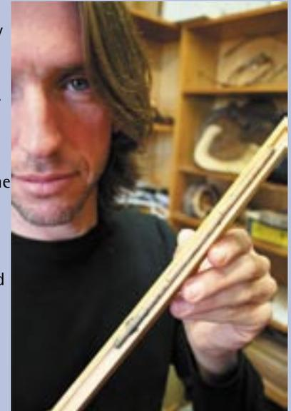
The cores are glued onto another piece of wood and then sanded down till they're mirror smooth and easily 'read'.
