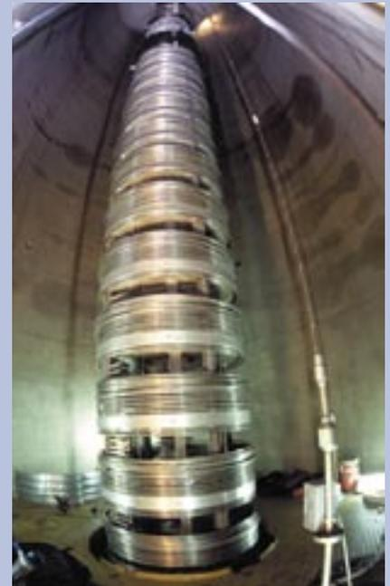
The Department of Nuclear Physics has devised an exercise in which students use the massive 14UD particle accelerator (part of which is shown above) to bombard an unknown metal foil with heavy ions to deduce what the foil is made of. Aidan Byrne tutors the students on the operation of the particle accelerator.
