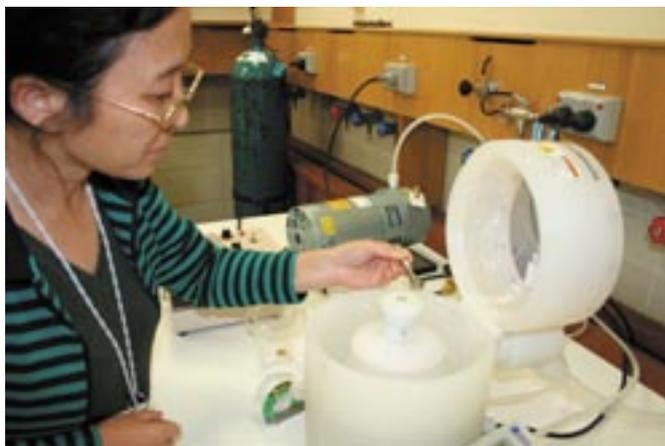
*Dr Yun Liu mounts a substrate on the spin coater. The spin coater is used to create thin layers (of around half a micrometre thickness) by dropping solutions of the material created through a sol gel process onto the substrate.*
