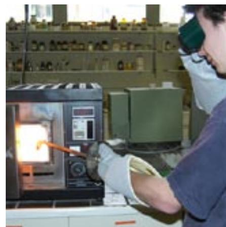
*Fire up the furnace: another ceramic sample is prepared in the synthesis lab of the Solid State Inorganic Chemistry Group at RSC.*
