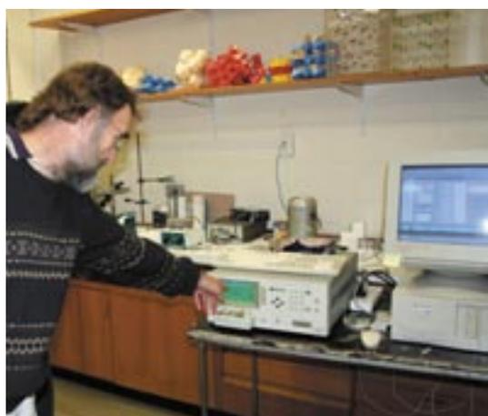
*Professor Withers with the LCR meter used to measure the capacitance of sample materials in order to determine their dielectric constant and dielectric loss.*
