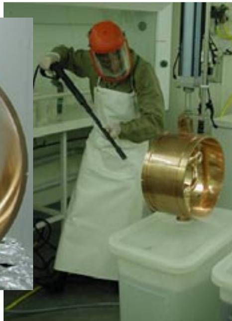
The resonators are made of pure copper and come in several configurations to accelerate different kinds of particles travelling at different speeds. To begin with, Dr Lobanov and his colleagues developed a system for coating the simpler quarter-wave resonators with niobium.
