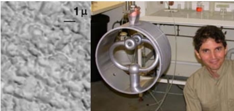
Dr Nikolai Lobanov with a lead-tin plated split loop resonator. When cooled down close to absolute zero this coating (seen under a microscope on the left) becomes superconducting.
