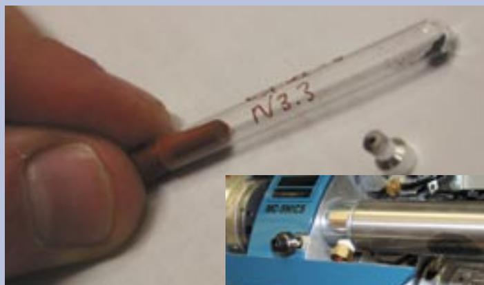
*The powder in the test tube is elemental carbon extracted from a sample. It's packed into a sample holder (below the test tube) and then loaded into SSAMS (right) along with many other samples. The sample wheel holds 39 samples.*
