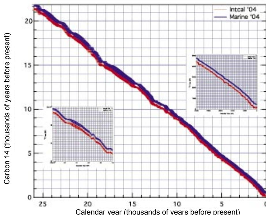
By combining a large number of datasets such as sampling from tree rings and sedimentary dating studies it's possible to create a calibration curve to correct carbon 14 age estimates to a calendar year. (Reimer, P et al 2004. IntCal04 Terrestrial radiocarbon age calibration, 26 - 0 ka BP. Radiocarbon 46, 1029-1058)
