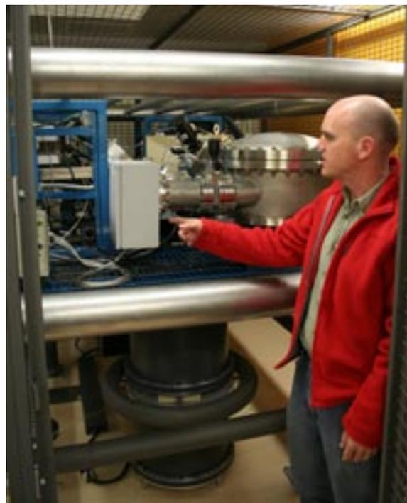
After being accelerated through the machine the different carbon atoms are collected and their ratio is estimated. Dr Fallon points at the carbon 14 detector.
