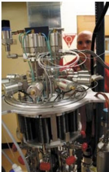
*An experimental rig for injecting the carbon samples as  $\text{CO}_2$  gas directly into SSAMS. This bypasses the need to use solid carbon and may transform radiocarbon research.*
