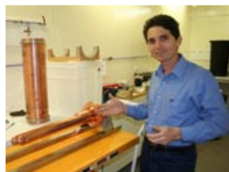
A prototype two-stub resonator half way through the machining process (left) and after machining (above).
