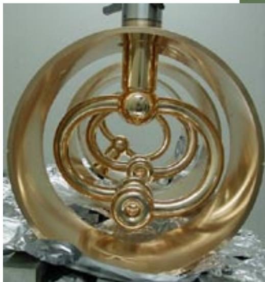
*Prior to plating the split loop resonators or polished and cleaned with high-pressure de-ionised water.*
