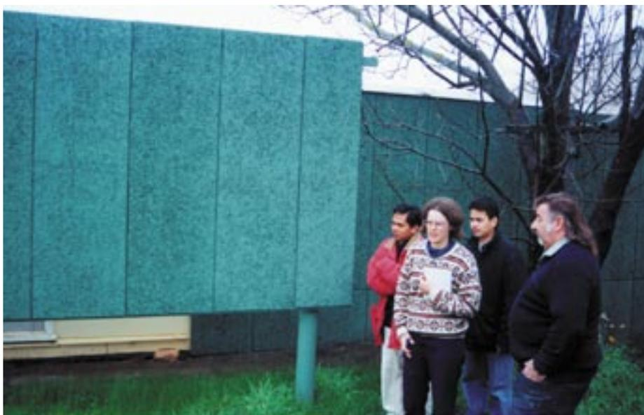
Innovative uses of wood-wool cement boards. Here they are being trialed as highway sound barriers (painted green). Pictured are (from the left) Rico Cabangon, Kate Semple, Mario Ramos and the Manager of WoodTex (Australia's sole manufacturer of wood-wool cement boards, based in Bendigo).
