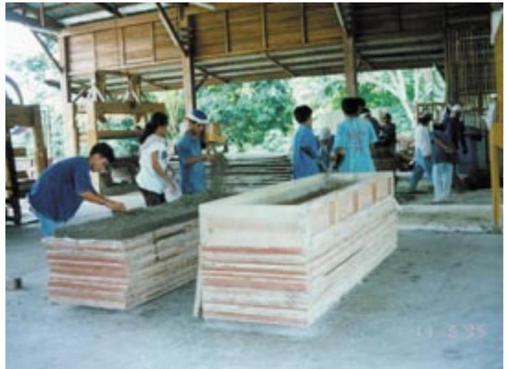
Wood-wool cement boards being made in the Philippines. Mat formation in fore ground, press left back and wood-wool cement mixer, right.
