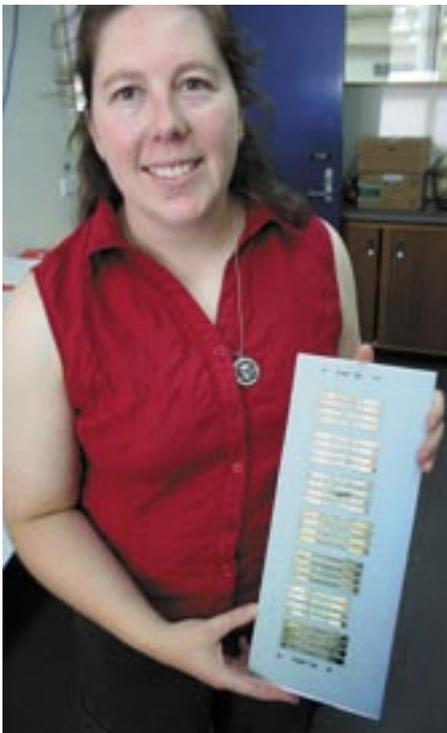
*Ms Procter with a set of silver samples stretched by the Department of Engineering's Instron machine to test the ductility of the various alloys.*
