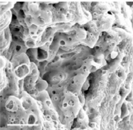
Scanning electron microscope images of the cavity floors shown on page 2. In the case of 150-fs pulse ablation (top) and 60-ps pulse (bottom). The 150-fs ablated floor is smooth, while the 60-ps one shows cavities and a “boiling” surface, indicating a lot of heat at the surface. The scale bars are 10- $\mu$ m long in both images.
