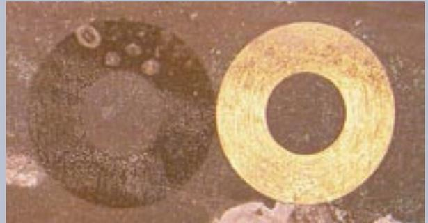
Brass coated with paint and wax after laser cleaning with varying energy levels. The experiment demonstrates the control over single layer removal achievable by appropriate selection of incident laser fluence
