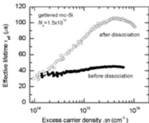
Lifetime measurements of silicon show significant differences for iron-boron pairs (bottom curve) and interstitial iron (top curve). This difference allow the amount of interstitial iron present to be calculated.
