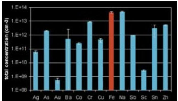
NAA results showing levels of different impurities in multi-crystalline silicon wafers. It's common for there to be between  $10^{13}$ - $10^{14}$  iron atoms in every cubic centimetre of silicon (shown in red).
