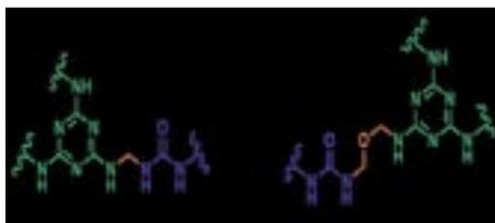
Possible products from melamine-urea-formaldehyde reactions: methylene linked co-polymers (left) and dimethylene-ether linked co-polymers.
