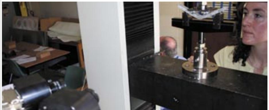
To analyse deformation in the aluminium foam composites Ms Styles used the ARAMIS strain analysis system. She first applied an increasing load onto the sample using the Instron. As it deformed, twin cameras (left-hand side of image) monitored its changing shape capturing stereo images of the deformation. Photogrammetric principles then track small correlation areas in successive images. ANU is the first Australian university to use the ARAMIS system.
