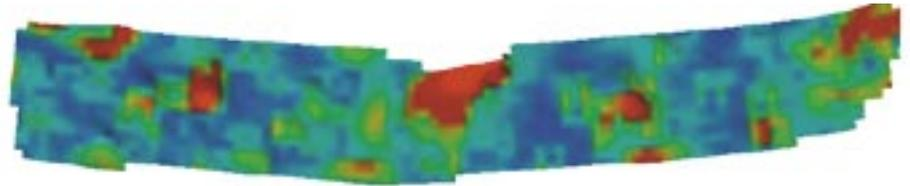
A strain distribution image produced by the Aramis system showing strain concentrations in the central deformation region as well as throughout the sample reflecting the cellular foam structure.
