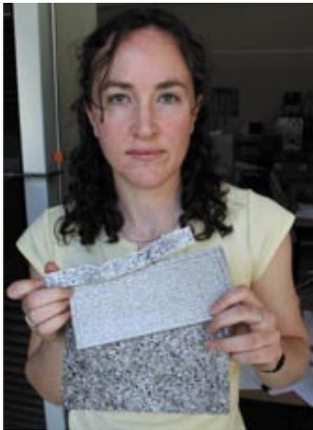
Milli Styles holds up three aluminium foam samples. The lower sample is a raw sheet of aluminium foam, the middle sample shows it with a coating of thermoplastic skin and the top sample is a section of the sandwich composite deformed from strength testing.
