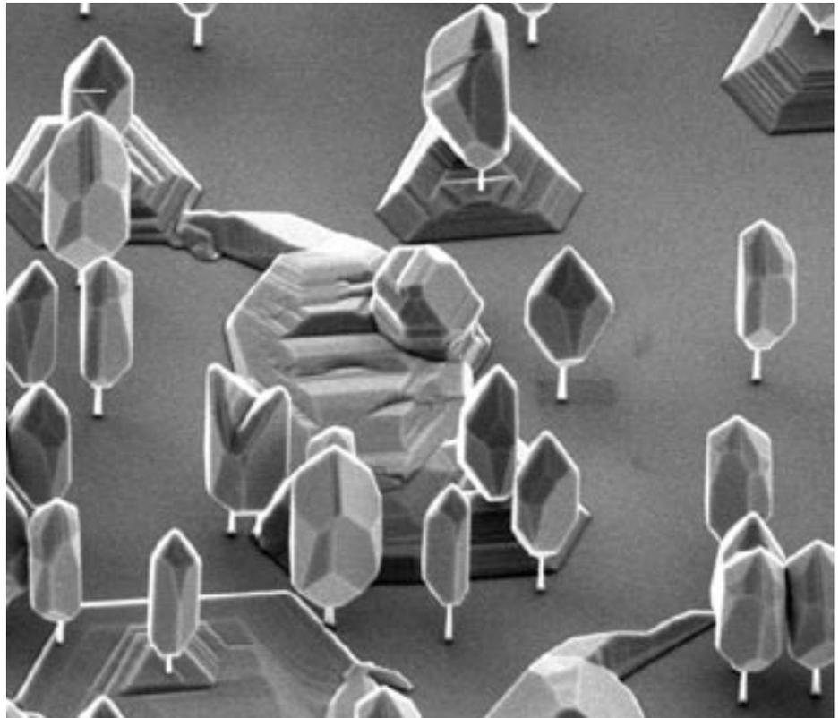
"That's because gallium antimonide has a larger lattice constant than gallium arsenide. When it crystallises on top of a wafer of gallium arsenide, large amounts of tension develop in the crystal structure of the gallium antimonide as the two crystal structures attempt to match. This tension prevents the gallium antimonide from forming smooth layers or growing into usable shapes.
