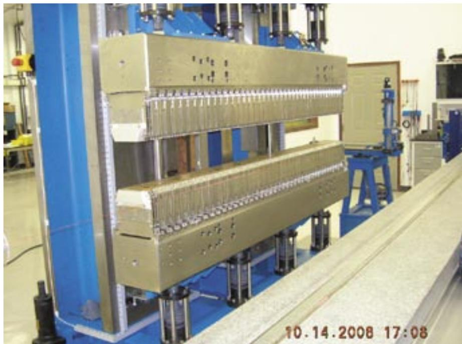
of periods (20 in this case) and the photon energies will be higher due to the increased magnet field (~1.9 T in the wiggler compared to ~1.3 T in the bending magnets). The result is 8.5 kW of output power and an enormous design challenge to direct photons of energies 4-45 keV from the wiggler onto the sample without melting either the beamline optics, the specimen under examination or the operator.
