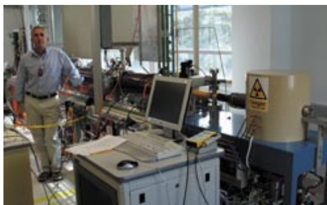
Professor Buckman with the positron beamline. The cylinder on the right houses the radioactive sodium 22, the source of the positrons.
