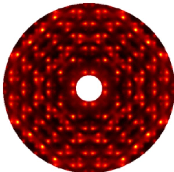
*The X-ray pattern of the diffuse scattering that occurs between the Bragg peaks for calcia-stabilised cubic zirconia (an advanced ceramic). Information contained in this diffuse diffraction is the key to understanding the nano-scale structure of this material.*
