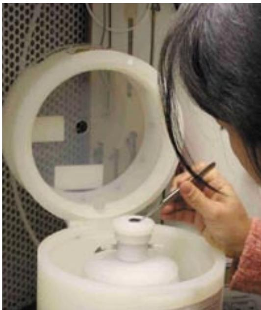
Dr Neto with a spin coater, a basic piece of lab hardware and almost all that's needed for the DIBIP process.
