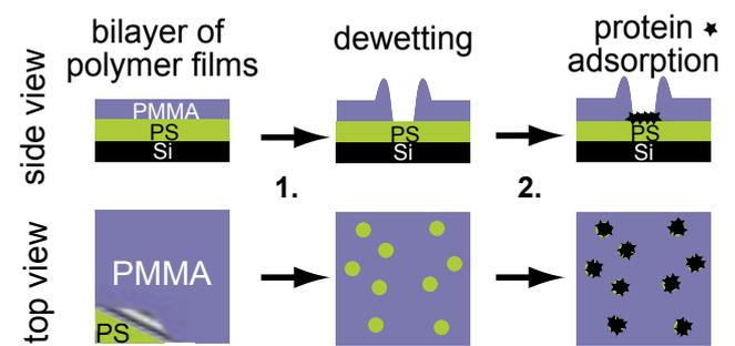
A schematic of the DIBIP micro-patterning method.
