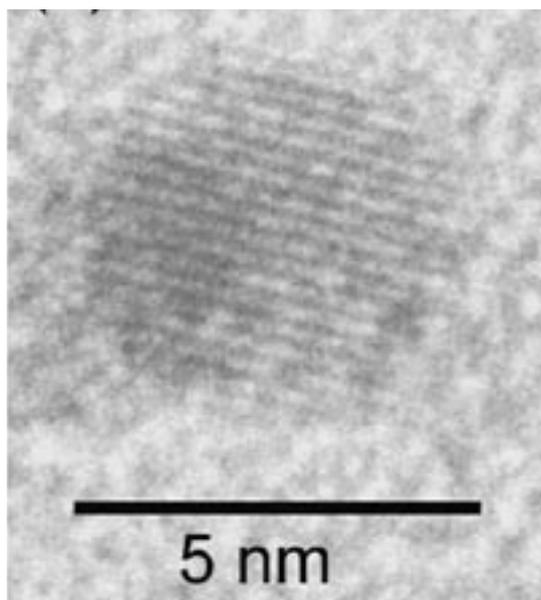
A high resolution transmission electron micrograph of a single gold nanocrystal. The lines represent rows of gold atoms sitting in a crystal array. To create amorphous nanoparticles of gold these nanocrystals are bombarded with high energy tin ions. As these ions pass through the nanocrystals they knock gold atoms out of their crystalline positions.
