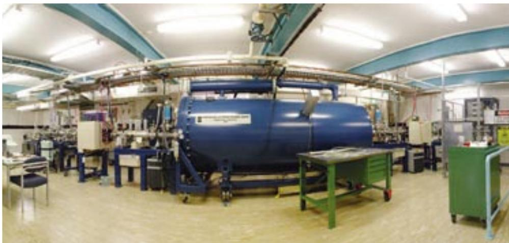
The high-energy, high-current ion implanter used to create and subsequently disorder the metallic nanocrystals. Negative ions are first formed in the source (far right), then accelerated, converted to positive ions and further accelerated within the accelerator (middle) and then finally rastered across the specimen within the sample chamber (far left). (Photo by Tim Wetherell)
