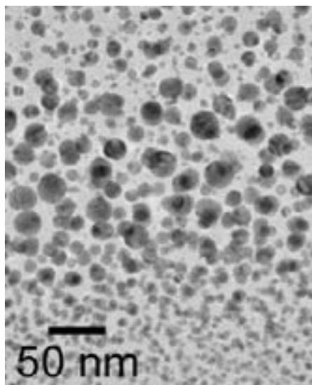
A transmission electron micrograph showing gold nanocrystals embedded in a thin layer of silicon dioxide (the scale bar represents 50 nanometres). The size and distribution of the nanocrystals are determined by the energy and number of gold ions implanted into the silicon dioxide, and the degree to which the sample is then heated (annealed).
