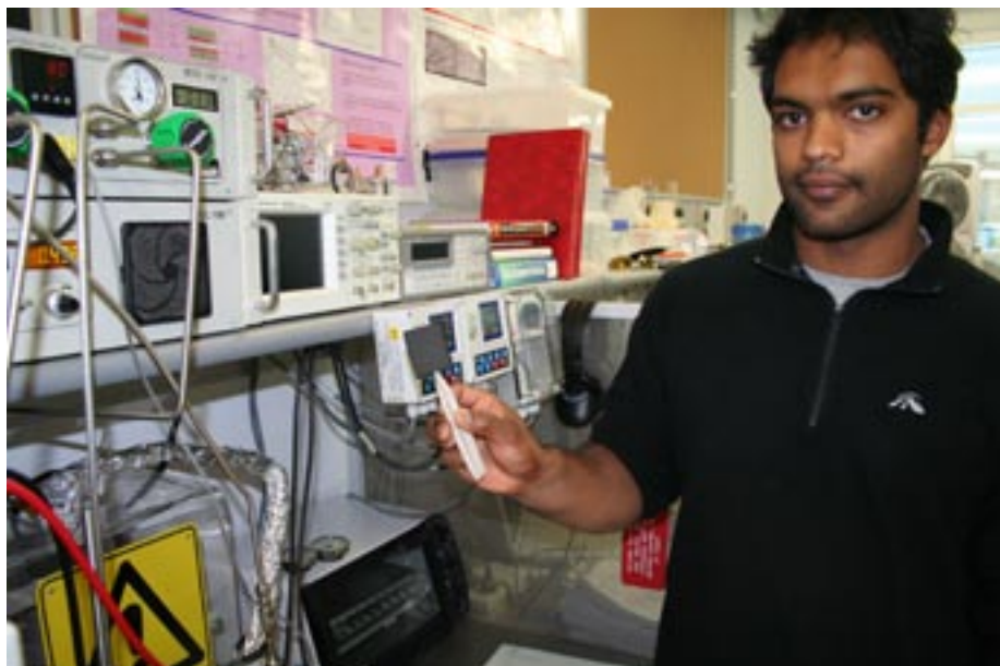
Devin Ramdutt holds a carbon electrode of a fuel cell that he has coated with platinum using plasma deposition. Besides running several plasma processing reactors, SP3 also maintains a fuel cell test station (behind Mr Ramdutt) to characterise the results of different treatments.
