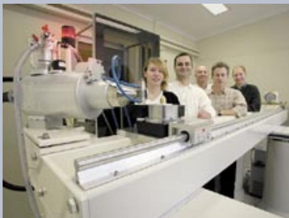
*The X-ray CT facility at Applied Maths - one of the few facilities in the world that can measure over three scales of magnitude simultaneously - from microns to millimetres. (Photo by Tim Wetherell)*
