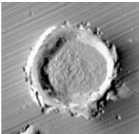
A scanning electron micrograph of one of the iron metal grains analysed from the lunar soil sample.
