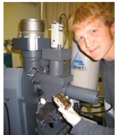
Ashley with the specimen holder for the SX100. Six samples can be loaded up for each run and samples must be coated in carbon to prevent charging from the electron beam.
