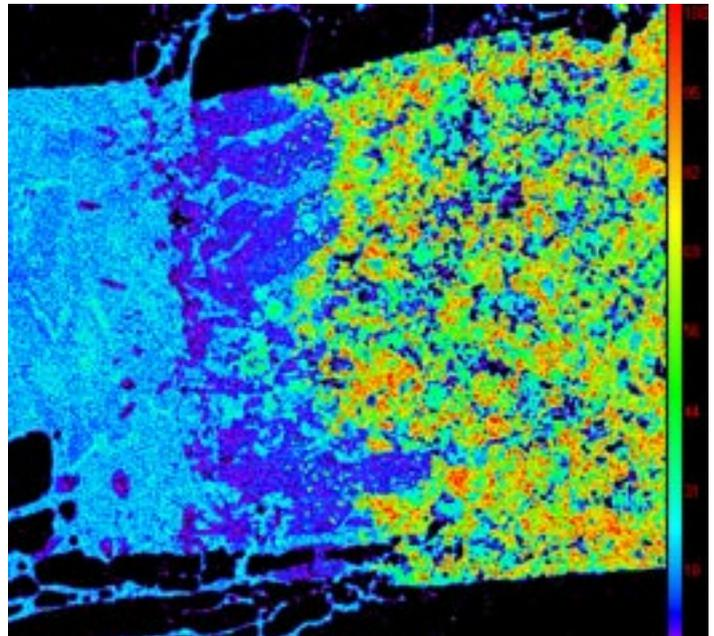
A map produced by the SX100 of calcium concentrations in a thin section of rock. The colours in the sidebar provide a guide to the x-ray intensity being measured. Roughly speaking, the greater the intensity the higher the level of calcium. Maps like this assist in identifying different minerals present in the rock.
