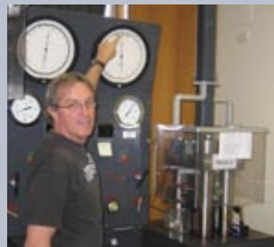
Greg Yaxley with the RSES high pressure rock presses used to synthesise olivine and garnet.
