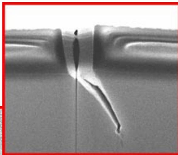
To study the cracks the researchers used a focussed ion beam to excavate a pit across the fracture (centre pic) and then a scanning electron microscope to image a transverse section of the crack (above). You can see how the crack goes all the way through the surface layer (about 1.2 micrometres deep) and then angles into the underlying silicon substrate.
