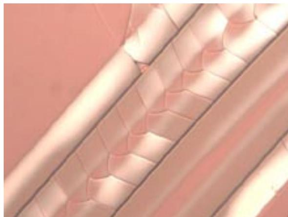
The researchers called the cracking pattern above 'snake skin' for obvious reasons. It's formed by two parallel straight cracks with repeated curved cracks in between. This form of cracking occurred relatively slowly, over several seconds. It could be observed happening by eye. The wavy cracks, in contrast, grow very quickly, too fast to observe.
