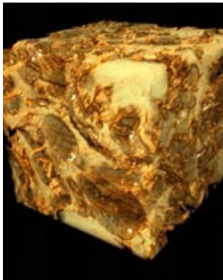
2. A computer tomograph of a small block of Mt Gambier limestone allows the three dimensional structure of the rock to be visualised.
