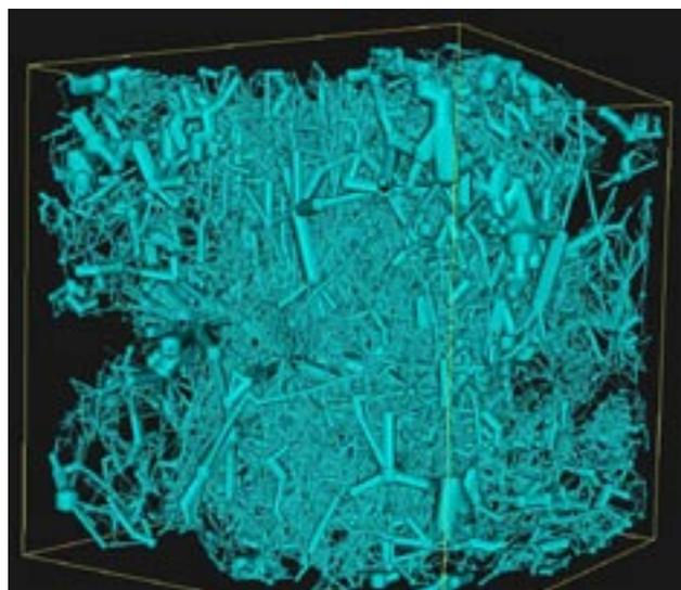
The topology of the pore space of a tiny sample (2mm cubed) of Mt Gambier limestone visualised at a larger scale to pictures below. Producing and manipulating data sets such as this requires enormous computational power and the use of sophisticated parallel algorithms.
