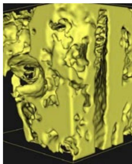
3. A tiny section of the tomograph shown in 2. The structure has been rendered to show the solid rock and the void spaces.
