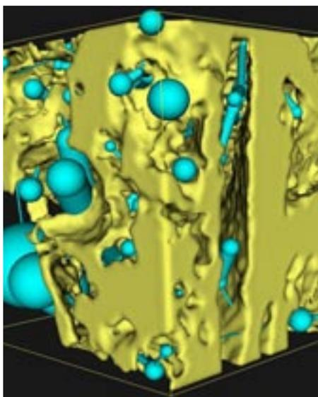
4. The pores and connecting passages are now modelled as balls and rods with the size of the balls reflecting the size of the voids and the size of the rods reflecting the size of the interconnections between the void spaces.
