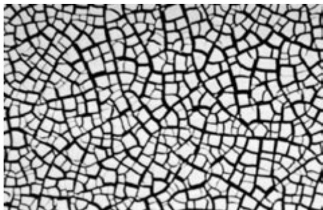
Crazy mud cracking patterns such as shown above (dried mud) and on the right (thin film of aluminium oxide) occur when materials experience isotropic stress. Clearly something different is happening with the thin silicon films.
