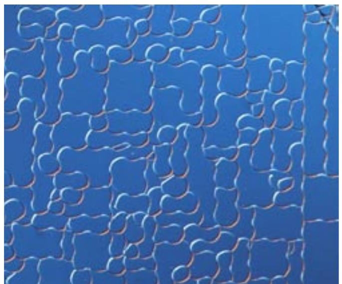
The researchers have observed many bizarre variants of the cracking behaviour. Pictured here is a form they have dubbed 'chain-mail' created from a network of interlinked wave cracks.
