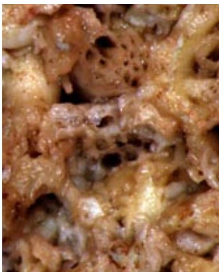
1. A close up of a fragment of Mt Gambier limestone showing fossilised remnants of the marine organisms from which it's composed. How do you make sense of such a complicated structure?
