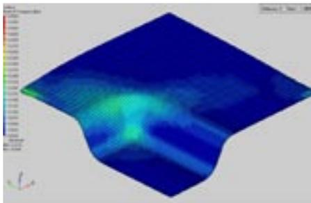
Upper image: FMLs using the composite Curv failed through a process of the metal skin cracking. Lower image: Computer simulation is used to model the process. Lack of wrinkling behaviour and high strain in crack-initiation regions correlate with experimental results.
