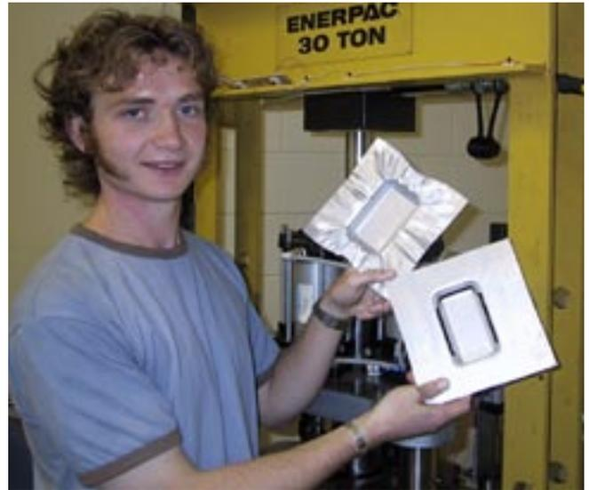
Luke Mosse holds up two test stampings of sheets made from different fibre-metal laminates. Both failed in different ways. The FML using Curv cracked, whereas the FML using Twintex crumpled.
