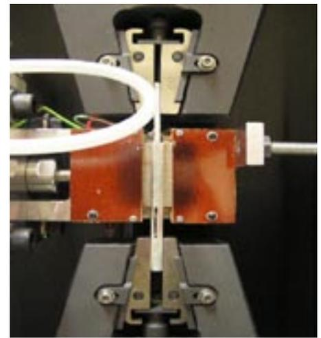
In order to measure the interfacial shear forces that exist between the laminate layers a special lap-shear apparatus was devised. Pictured above, this apparatus allowed the shear force between the middle composite layer and the metal layer to be measured simultaneously with temperature and external pressure (stamping pressure) on the FML.
