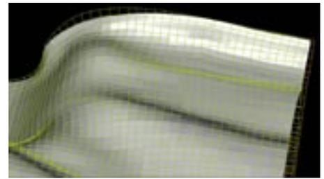
Upper image: FMLs based on Twintex failed by wrinkling (a completely different behaviour to the Curv-based FMLs). Lower image: The model for this system (the wire mesh = aluminium and grey = composite) also displayed this behaviour.
