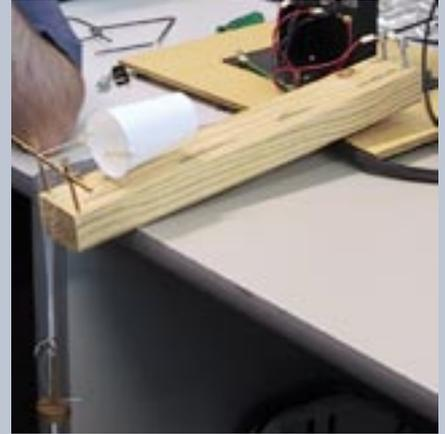
“We've tested this approach in a device called a pantograph. The pulleys attached to the SMA wires control the movements of two connected robot arms. The contraction of the SMA wires is controlled by measuring the electrical resistance in the SMA wires. We've demonstrated that this approach allows for movement significantly faster than has been achieved by any other system.”
