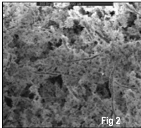
Figure 1 is a scanning electron micrograph showing the fracture face from a raw clay sample at 100X magnification. The surface reveals the presence of numerous voids that are randomly distributed, as well as particles of varied size and distribution. When paper pulp is incorporated into clay, the heterogeneity of the material is enhanced considerably as seen in figure 2. The paper fibres are not only randomly distributed through the matrix but also randomly oriented.
