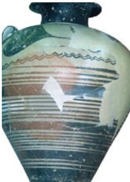
Paperclay is a composite ceramic material made by the addition of paper pulp to any type of unfired clay. Conservators at the National Gallery of Australia together with materials researchers at ANU are testing paperclay to see if it might make a suitable gap filler to compensate lost sections in earthenware ceramics.
