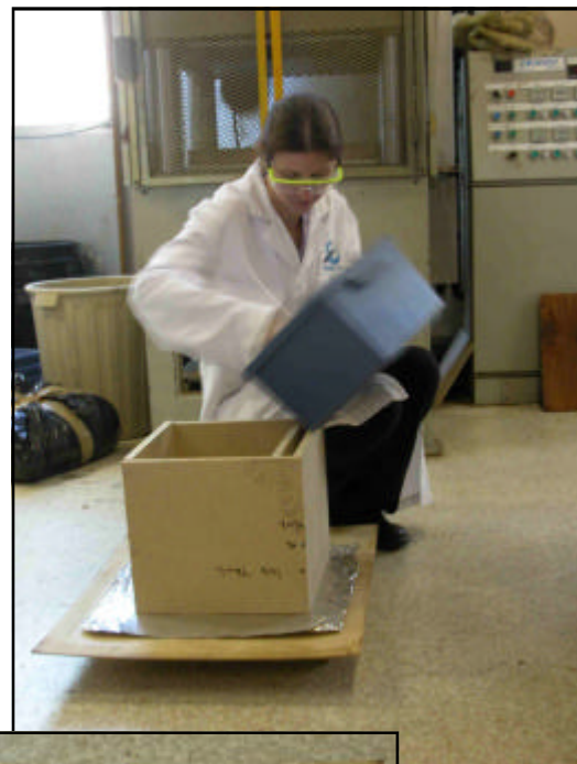
Olivia adds resin blended flakes into a wooden frame. This produced a mattress, suitable for pressing. ▶▶
