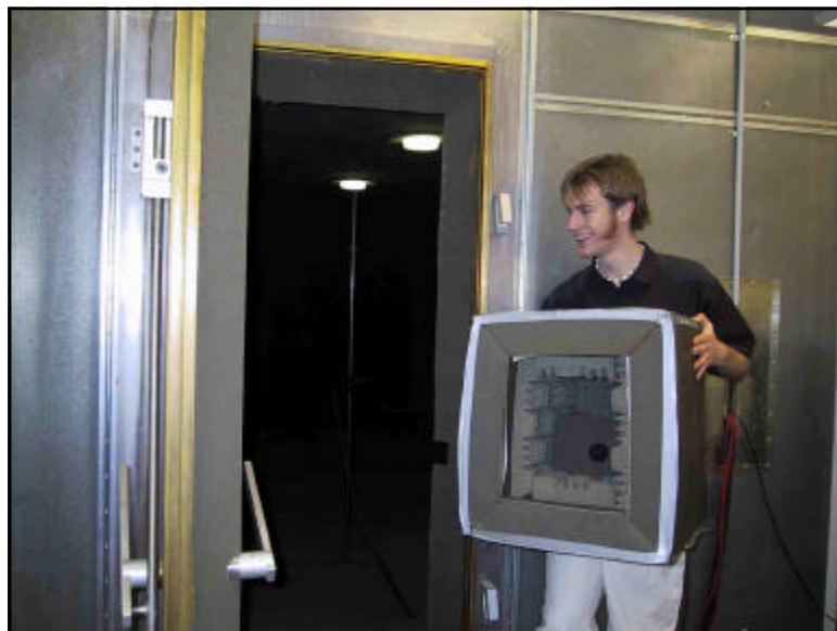
▲▲ Matt Curtis prepares to take his mini anechoic chamber into the quiet room. Note how thick the foam is on the door into the chamber.
