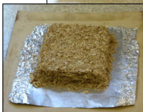
◀◀ A mattress of unpressed wood particles
