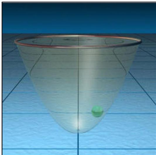
▲▲ Optical tweezers trap small particles in an imaginary valley or potential well. The further it moves away from the centre, the stronger the force pulling back. (Graphic by David Carberry)
