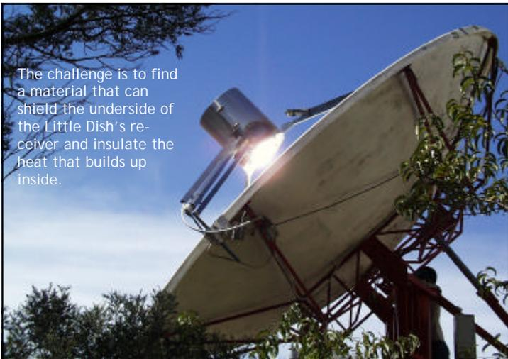
The challenge is to find a material that can shield the underside of the Little Dish's receiver and insulate the heat that builds up inside.
