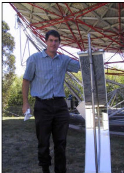
▲▲ Keith demonstrates how their system of attaching the new low-iron glass mirrors to metal creates mirrors that can bend.
