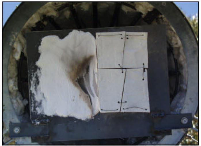
▲▲ The commercial sample on the left next to Tony's new ceramic on the right. (Note, these samples are sitting over a hole in the bottom of the receiver through which the concentrated sunlight normally passes.
