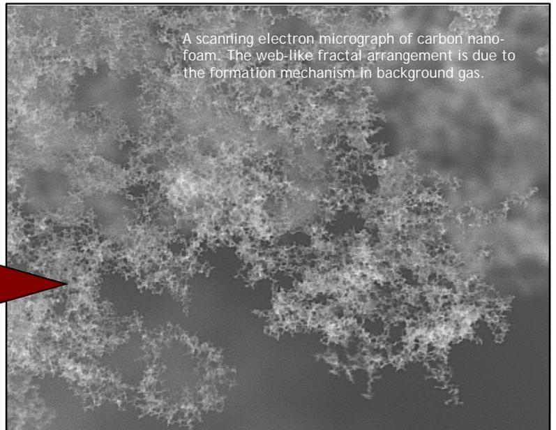
A scanning electron micrograph of carbon nanofoam. The web-like fractal arrangement is due to the formation mechanism in background gas.
