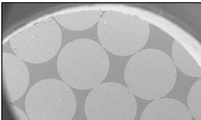
▲▲ A cross resection through the BMG rods. The circles are tungsten wire
