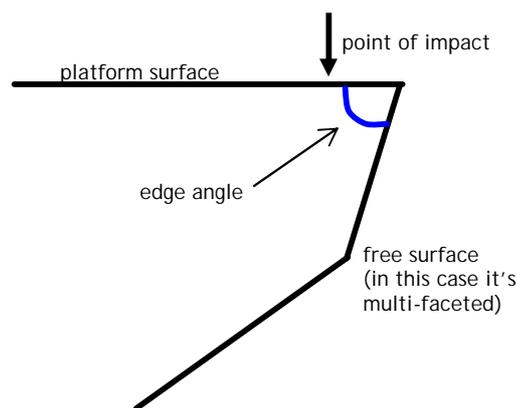
▲▲ Figure 1: the two most important factors in determining the mass of a resulting flake are the thickness of the platform and the edge angle
