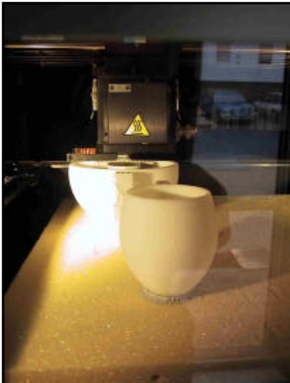
▲▲ An object being created within the FDM8000. Prototypes are constructed by building them up layer by layer.
