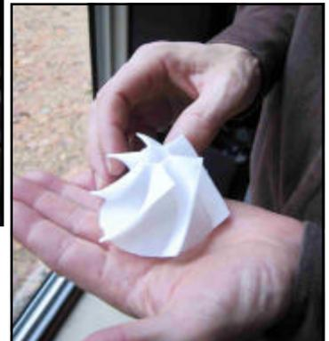
▶▶ A prototype turbine created by the FDM8000.
