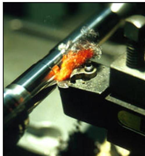
▲▲ Cubicom machining hardened tool steel. It's high thermal stability means no coolant is necessary.
