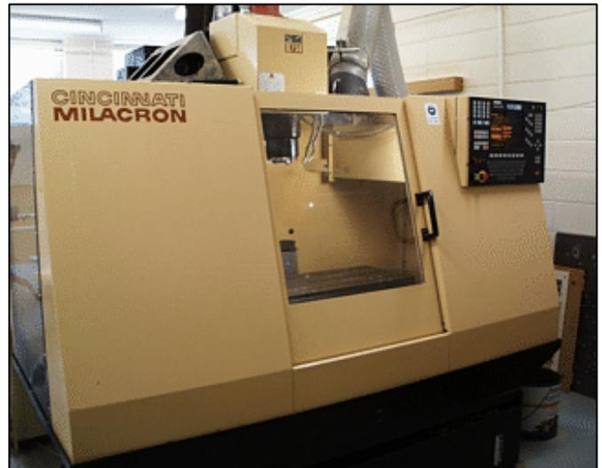
▲▲ The computer controlled CNC apparatus can produce parts made to measure. It forms part of the Advanced Manufacturing lab.
