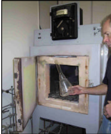
▲▲ Items produced during the day are heated in an annealing oven overnight.
