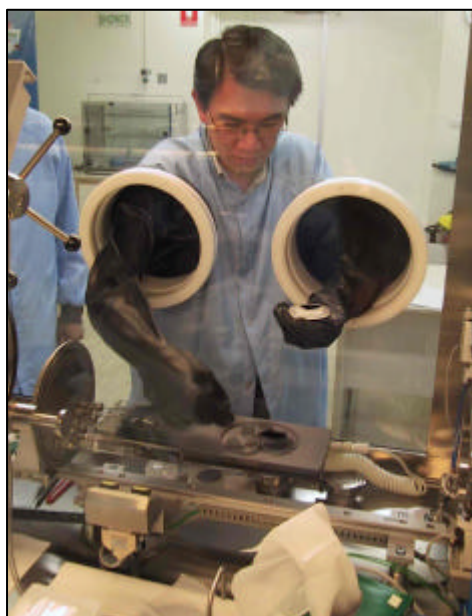
◀◀ Dr Hoe Tan prepares a wafer ready for insertion into the new MOCVD reactor.
