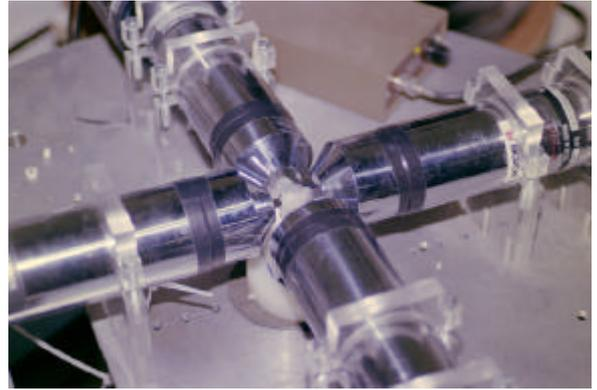
▲▲ An array of four barium fluoride detectors are used to detect radiation from the probe nuclei.
