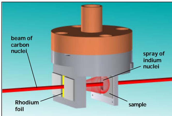
▲▲ Implanting radioactive nuclei into a semiconductor sample involves striking a thin rhodium foil with a beam of carbon nuclei to generate radioactive indium nuclei. These spray out of the back of the foil and become lodged in the semiconductor sample mounted behind the foil.
