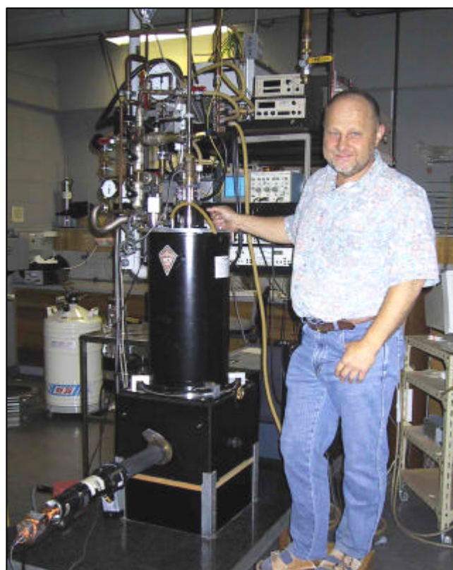
▲▲ Elmars with an older version of an MCD spectrometer. The next generation device is expected to produce powerful new insights on the nature of metals in metalloenzymes.
