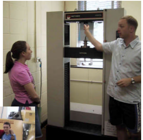
▲▲ Paul Compston measures the strength of one of the student's hairs. Human hair, weight for weight, can be as strong as
