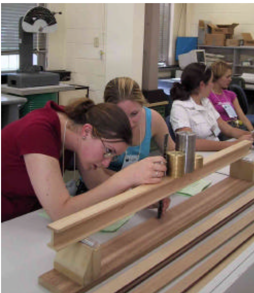
▲▲ Students measure the stiffness of pieces of wood in a variety of configurations.
