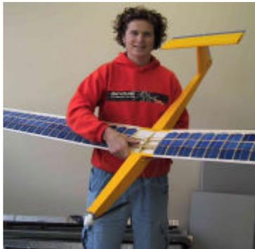
As is often the case, it's often the simplest solutions that are the best. It was decided early on in the project that the majority of the aircraft would be built from balsa wood, which has one of the best strength to weight ratios available. To add additional strength and rigidity to this frame, a heat-activated (yellow) shrink film was used as a skin on the balsa wood. The wing containing the cells is covered in a transparent film.
