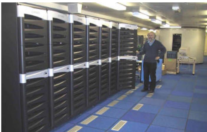
▲▲ Dr Bob Gingold, Head of the ANUSF, stands next to one of three banks of Compaq processors that comprise the ANU supercomputer. In total there are 120 processes linked to form a supercomputer with a peak speed of nearly 1 teraflop, with total memory of nearly 0.5 terabytes, and total disk storage of over 10 terabytes. Behind Bob (to the right) is the robot driven tape library that serves as a mass data storage system.
