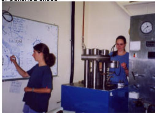
The Piston-cylinder apparatus in the High-Pressure Laboratory.
