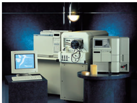
▲▲ The VG Quattro II, one of the many mass spectrometers available at the ANU MS.
