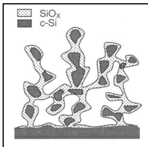
Schematic diagram of porous silicon showing small crystalline regions with dimensions less than ~10 nm. This material exhibits strong room-temperature photoluminescence due to quantum confinement of carriers in these nanometre -sized regions.
