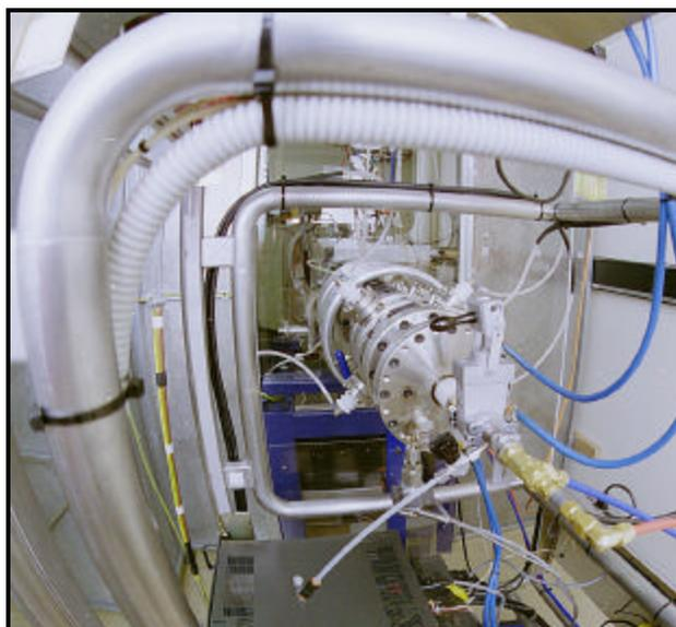
The ion source in the low energy ion implanter used by EME to fabricate Si nanocrystal materials.
