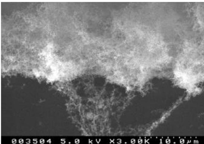
Scanning electron micrograph of the carbon nano foam, a novel material built using ultra-fast pulsed laser deposition.
