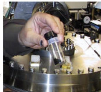
However, for all its advantages, there are several technical obstacles that stand in the way of its widespread commercial use. Its main drawback has been the deposition of particulates on the film resulting from inhomogeneities in the material being vaporised by the laser. These particles produce a lumpy film of uneven character.
