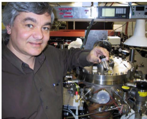
Dr Andrei Rodes with a vial of carbon nanofoam in front of the equipment that produced it. (Vial seen in more detail in top right corner.)
