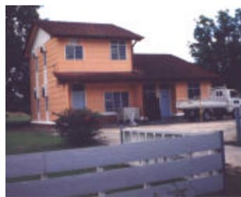
Not only is the house built of cement-bonded particleboard, so is the front fence.
