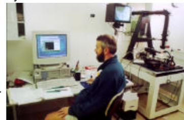
Laser-ablation ICP-MS analysis in progress. The sample cell is on the right.
