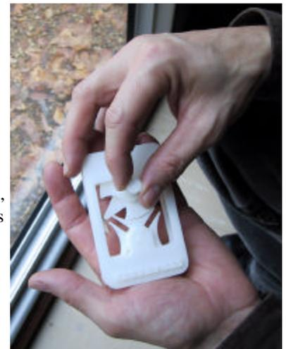
With an upgrade the FDM8000 can build models with moving parts and cogs that don't need assembly.
