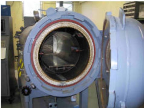
◀ The autoclave used by the Advanced Materials Lab to produce high tech composites.
