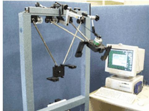
◀ The Dinkum Impact Tester used measure the impact damage on composites.
