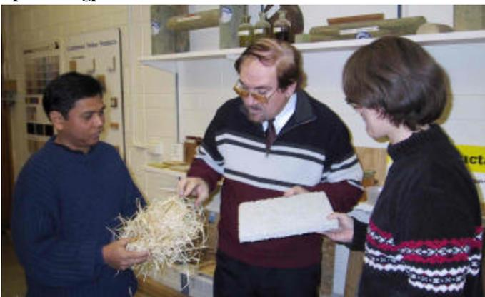
Rico Cabangon (left) and Kate Semple show Dr Patto (centre) a wood-wool cement board and the raw wood fibre from which it was made.
