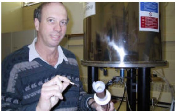
Max Keniry with a 5mm zirconia rotor that holds the solid sample.
