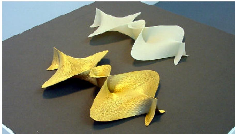
*ABS polymer products of the FDM8000 rapid prototyping machine. The lower artefact has had a thin gold deposition added post-processing. Designed by Gilbert Riedelbauch, Lecturer Applied Design, Computer Art Studio, The Canberra School of Art.*
